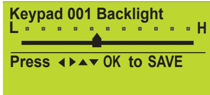
2. Use the [←] and [→] keys to adjust the bar until the desired backlight is reached.
